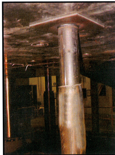
The Ball Buster Prop after 450mm of stable closure.
